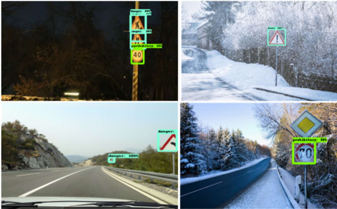
Figure 12: Traffic sign detection and classification in bad visibility conditions (night, snow, truncation)
