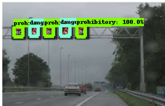
Figure 13: Digital traffic sign detection and classification
