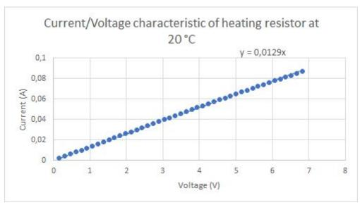
The graph above shows the current/voltage characteristic of the heating resistor (polysilicon) at 20  $^{\circ}$ C, the resistance is 77  $\Omega$ .
