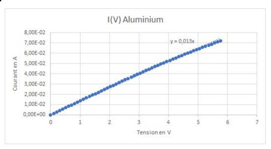
The graph above shows the current/voltage characteristic of the temperature sensor (aluminium) at 20  $^{\circ}$ C, the resistance is 77  $\Omega$ .
