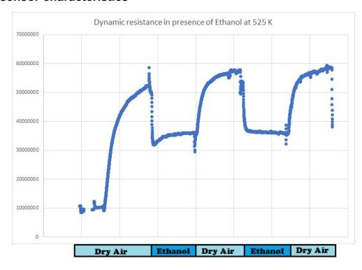
In order to determine the gas sensor characteristic, the resistance evolution is measured in presence of different gases. In the case of a resistance drop, that reveals gas presence and the gap observed is proportional to the concentration. The time response is the parameter used to determine the nature of the gas.
