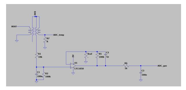
Above is the typical application of the sensor we built, with an analogical circuit. in order to be able to read the gas value we have to amplify the sensor's output. For the amplification we recommend using the LTC1050 with the analogical system described above. The tension from the ADC\_gas label can be connected to a 5V ADC, like an Arduino. The tension to heat the sensor should be up to 10V during the measurement.
