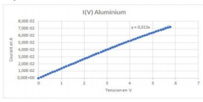
We can see on this graph that when the current/voltage characteristic of the temperature sensor (aluminium) is at 20 °C, the resistance is 77 Ω.
