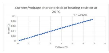
We can see on this graph that when the current/voltage characteristic of the heating resistor (polysilicon) is at 20 °C, the resistance is 77  $\Omega$ .
