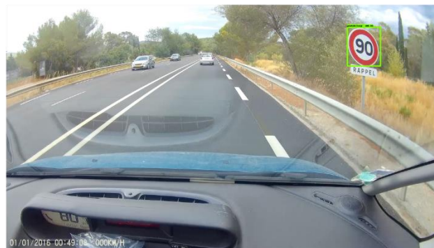
Figure 11: Traffic sign detection and classification using RFCN-Resnet 101
