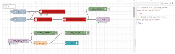
For example, for a value greater than 250 lux, we established that the led would be green, otherwise, it would be red. If we give 100 lux as the light value, the result, as it should, is:
