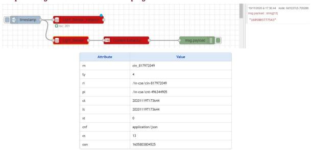
As we can see in the pictures above, we created a value using the ContentInstance, and visualized it using the Content Extractor linked to the Sensor, here the Ligh\_Sensor. We could verify the data was correct, using the OM2M web page created in Lab 3.
