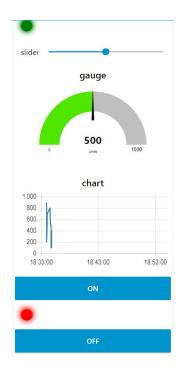
In this dashboard the slider sends a light value to the light sensor, to simulate a light variation. The first led shows if the light values are above 250 lux or note.
